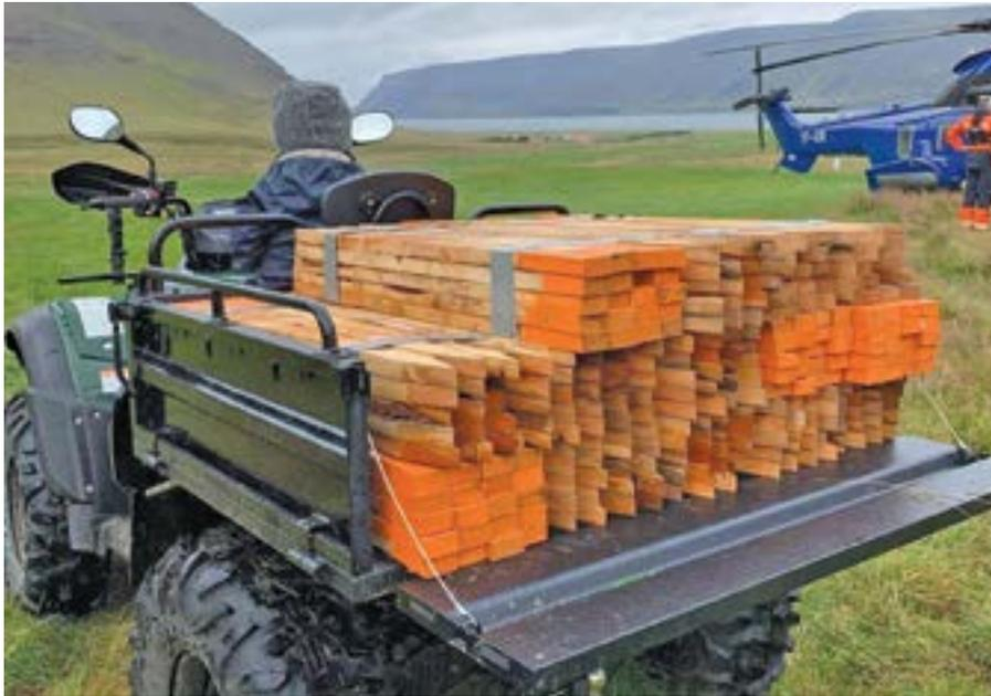
The TGB Blade 600 AR EPS 4x4 is ideal for commercial use, and comes equipped with a cargo bed that can carry a useful load of up to 200kg. PHOTOS: SUPPLIED
